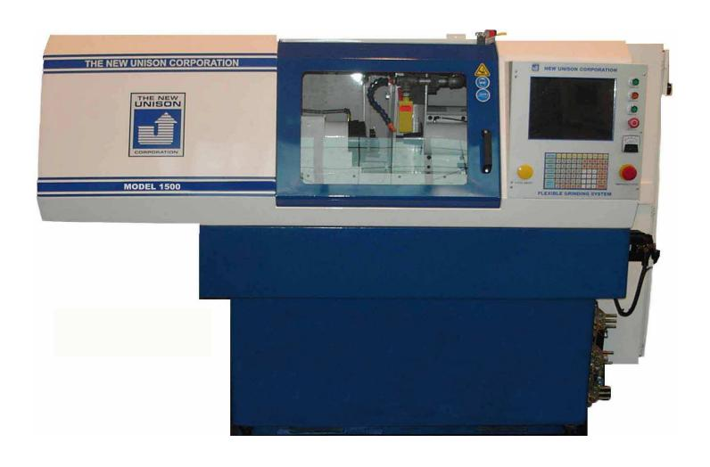
**UNISON MODEL 1500 CNC PROFILE GRINDER (PunchMaster)** features a polymer cast base and new software. The design of the base provides significant dampening properties to absorb vibration during grinding. The improved base increases accuracy during grinding as well as the surface finish on the parts. Polymer bases are less sensitive to temperature fluctuations due to a lower thermal expansion coefficient thus improving precision and increasing productivity.
