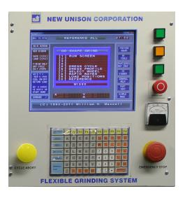
Our latest Version 7 software tool grinding technology utilizes the new Windows 7<sup>TM</sup> Operating System. The combination of this software package, allows the Model 1500 to meet the most demanding grinding applications with faster cycle times. Unison's Parametric Control allows the operator to program parts by means of a simple menu both quickly and efficiently.
